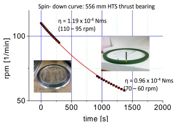
Fig. 4. Spin-down curve of the CMB superconducting bearing at LN<sub>2</sub> cooling. The degree of rpm decay depend on the magnetic inhomogeneity of the PM ring  $\Delta B$  which causes magnetic hysteresis and eddy current effects. The non-linearity of the curve arises from ambient pressure air drag.
