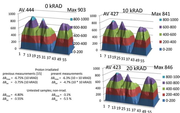
Fig. 5. Scanning trapped field profiles before and after proton irradiation. The water equivalent dose of 10 krad corresponds to an expected 5 years stay at the Sun-Earth Lagrange point two (L2) under cosmic ray environment.
