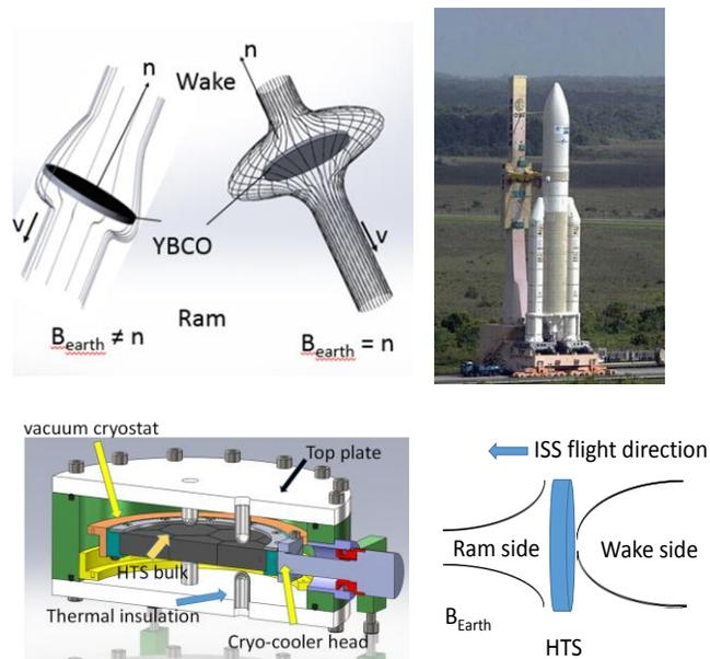
Fig. 1. Concept of YBCO bulk investigation under space conditions. Particle impact control by trapped flux measurement and conductor interaction with Earth magnetic field  $B_{\text{Earth}}$  running in Magvector/ MFX experiment since 2014 at the ISS.
