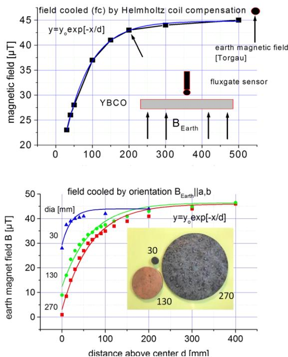
Fig. 6. Earth magnetic field shielding experiment with a 110 mm x 12 mm YBCO plate (top) and size variable shielding performance (bottom). The flux gate Hall sensor FC 100 was each time in central position and detected the Earth magnetic flux shielded by the HTS plates at 77 K.
