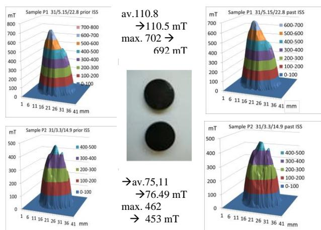
Fig. 2. Comparison of trapped field measurements of two 30 mm YBCO single crystal samples of thickness 3 mm (lower bulk) and 4 mm (top position). The samples were transported to the International Space Station (ISS) with the German mission “blue dot”, stored in the ESA Columbus laboratory and returned 5 months later with the astronaut A. Gerst. The values describe parameter prior mission → parameter after returning.
