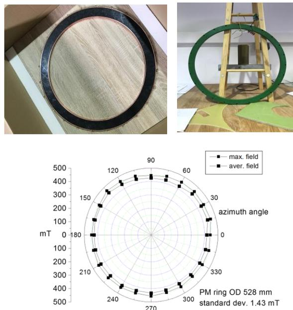
Fig. 3. Large HTS magnetic bearing (D=560 mm) for cosmic microwave background (CMB) polarization modulator consisting of YBCO stator (top left) and PM rotor (top right) together with the measured magnetic homogeneity of the PM ring (bottom).
