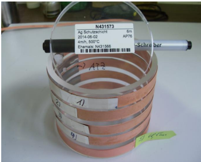
Fig. 2. Experiments of copper plating parameters on CC surfaces: Substrate Hastelloy and NiW, plating solution, current density, and pulse structure.
